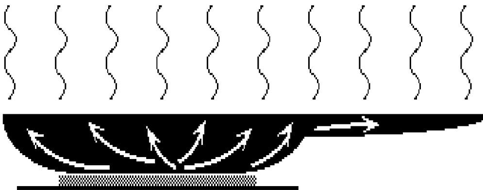
**Figure 5. Heat conducted through the pan to handle**
